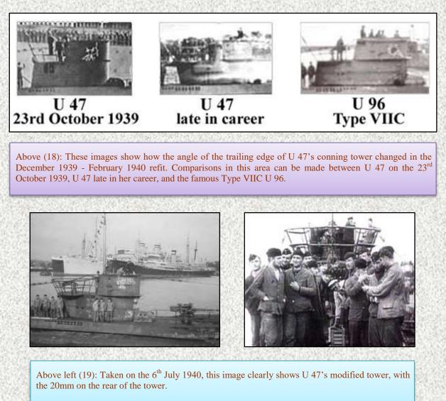
Above right (20): Another 6<sup>th</sup> July image, this photo illustrates how the new tower railings protruded out much farther than the old style tower railings.
