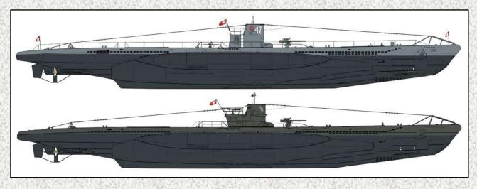
Above (30): U 47 at the start and end of her career, with the lower hull paint being *Schiffsbodenfarbe III Grau* (RAL7016).
