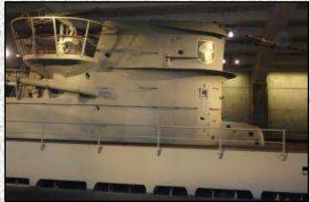
Above (16): This clear image shows the colour of the paint used upon the upper hull and tower of U 505 at MSI. The green shield background of the shell emblem can also be seen. Several holes punched in the side of the tower were caused by aircraft and vessels belonging to the task force which captured U 505. The tube at the left hand side contains a spare barrel for the 37mm automatic. Lastly, note how the deck railing stops abruptly just ahead of the magnetic compass housing. Originally this railing had an additional three vertical stanchions. (Ernest Roth)
