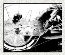
Above left (1): Although this image is of the VIIB U 86, it provides a very good view from the rear of the typical wooden floor fitted to most Type VIIC U-boats.
