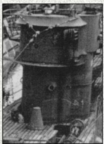
Of the 35 VIICs and VIIC/41s which have been observed in photos, only six (17%) retained the standard magnetic compass housing by the end of hostilities. This suggests that the majority had been converted to the Askania type by the end of the war.
