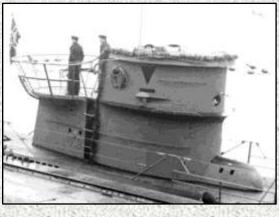
Above (6): The standard magnetic compass fairing on U 408. As the photo illustrates, the fairing abutted the front of the tower.
