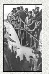
Left (D12): The very low height of the tower can be seen in this photo in which the top of the bulwark only comes up to chest height. It is easy to appreciate why the curved railing bars needed to be added above the tower.
