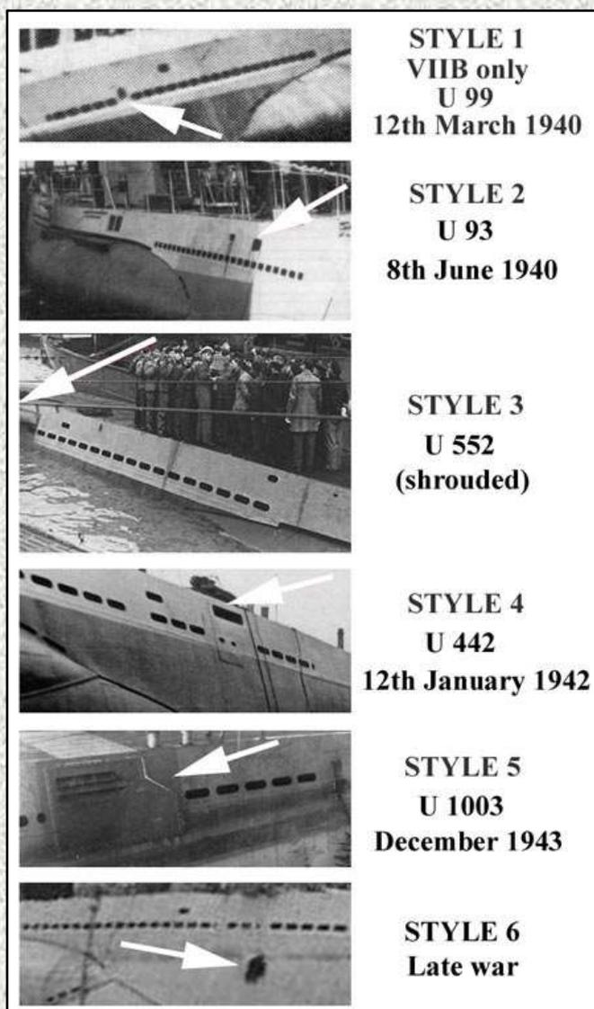
Left (54): The various styles evidenced in photographs of Type IXs, with the right hand side being the front of the boat. For simplification, all styles here use a quarter vent ahead of the exhaust outlet rather than a half vent. As discussed in Part VII, this vent size differed between boats.
