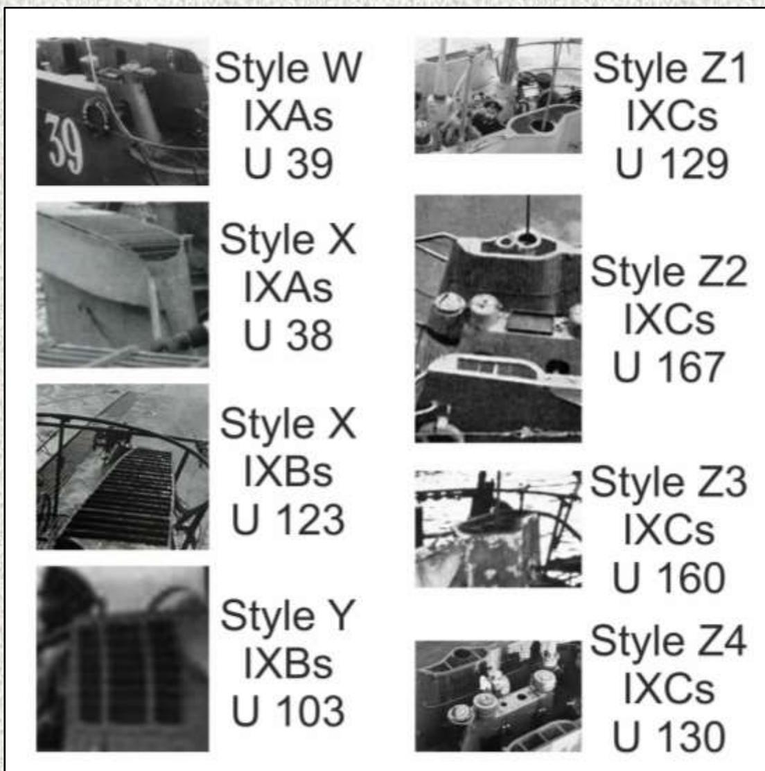
Above (5a-5h): The various styles of air intakes on Type IXs. Given are the sub-variants each style was applied to and the individual U-boat shown in each photo. Style Z3 on the **starboard** side was very similar to Z4.
