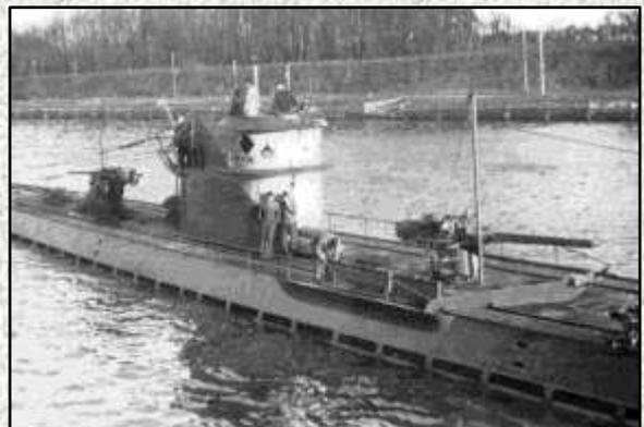
either side of the top of the hull around the area of the 105mm gun (Revell parts 82 and 83). Although the shape differed from the version fitted to the VIIIs, this first type fulfilled a similar function on the IXs by helping to prevent waves from crashing over from the sides of the hull. The second type - referred to as the deck breakwater - was the shield fitted across the deck directly ahead of the 105mm gun; this helped to reduce the water coming at the crewmen from ahead.
