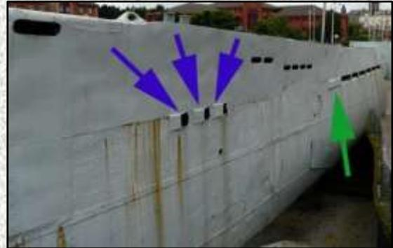
Above left (70): The rear section of a dissected U 534 at Liverpool. Although the pole obscures this area, we can still see that the quarter-length vent (Q) is ahead of the exhaust outlet area. There is a half-length vent (H) behind where the exhaust outlet would have been. In earlier IXs there were four main vents in position P. In this photo we can see that U 534 had two main vents, with six shrouded vents (shown with the pink arrows) in place of the rear two vents in position Q.
