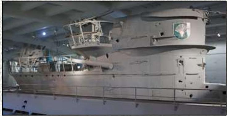
Right (96): U 505 under cover in Chicago with a Turm IV tower which replaced the boat's Turm II.
