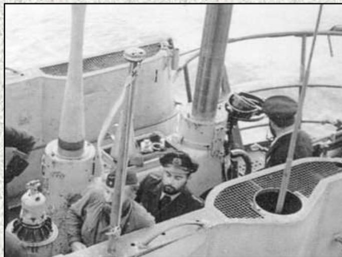
Above (7): Style Z1 on U 129 in April 1942 clearly shows the criss-cross mesh grill and the periscope rod aerial in the raised position.
