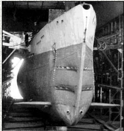
Above (34): The two vents near the top of this unidentified boat indicate to us that it is a Type IXC. Clearly there is no S-Gerät on the stem of what could be a later war boat.
