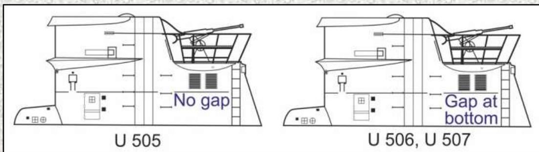
Above (14): As covered earlier, there was a difference in respect to the two grills lower down. On the IXAs, IXBs and the *Deutsche Werft* IXC U 505, there were eight horizontal bars arranged with equal distance between the bars and no gap at the bottom. From U 506 onwards, the number of bars was the same but a significant gap appeared beneath the lowest bar.
