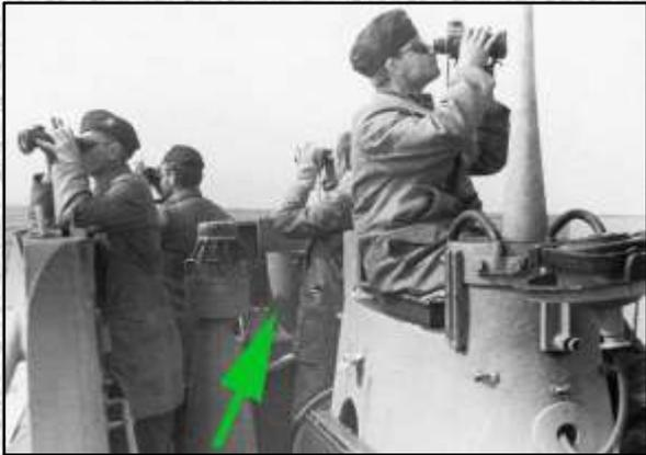
Left (22): An early photo of U 124 before the windscreen baseplate was added. The green arrow points to the position of the vertical tube housing the third periscope. Note the foldable step at side of the periscope housing and the extended periscope at the rear having no anti-vibration wires; these features point to an early time period after being commissioned in June 1940.
