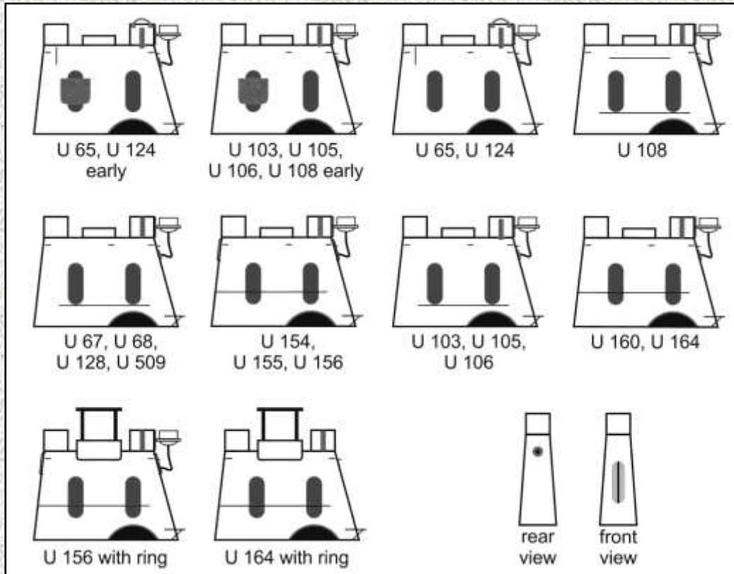
Above (32): The periscope housing on a range of IXBs and early IXCs showing many of the features discussed in this section. The foldable metal seats, as seen on the two profiles at the top right, were on the IXAs and early IXBs. A lot of features are missing from the Revell kits such as the large semi-circular gap, grips, C-shaped step, small loops, vertical plate and oval gap at the front of the housing.
