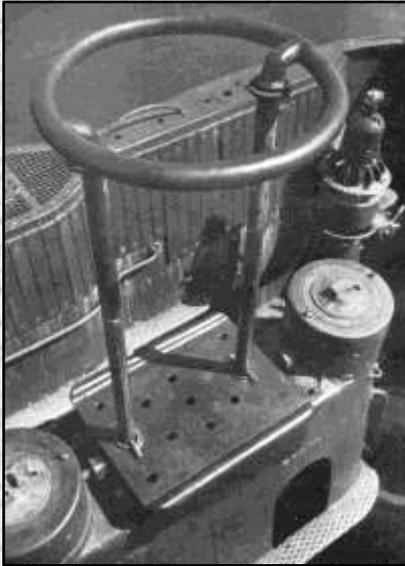
Left (33): The support ring can be seen in the extended position on U 156 in August 1942. Other features are the ledges with criss-cross pattern, periscope lids, wooden panelling on the bulwark sides, early UZO and semi-circular grip bar ahead of the air intake grill.
