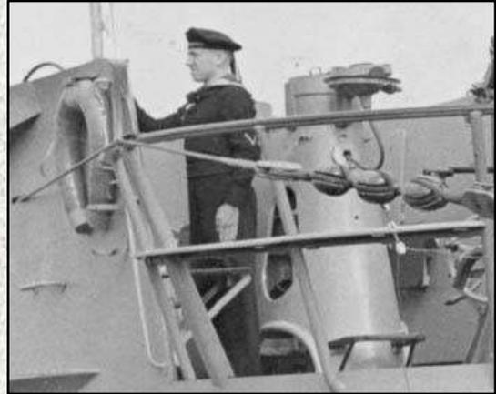
Above (31): The commissioning of U 103 in July 1940. The semi-circular drainage gap at the bottom of the periscope housing can clearly be seen along with a substantial rim at the edges. The C-shaped ring and two support bars below can be seen at the bottom of the rear end of the periscope housing.
