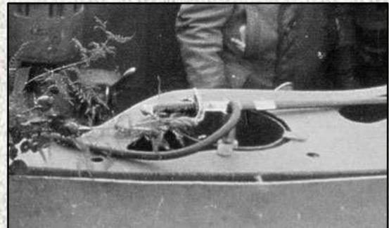
Above (19): Although partially obscured by flowers added to the tower at the conclusion of a patrol, we can see part of the mystery object on U 123. The cable is secured into the top of an object which is itself fixed into the middle of the vertical tube.
