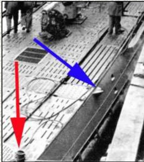
Above (39): U 108 on the 26<sup>th</sup> November 1942, with this feature in position 1. The blue arrow points to the fairlead and the red arrow points to the bollards. Clearly there is plenty of separation between the fairlead and bollards.
